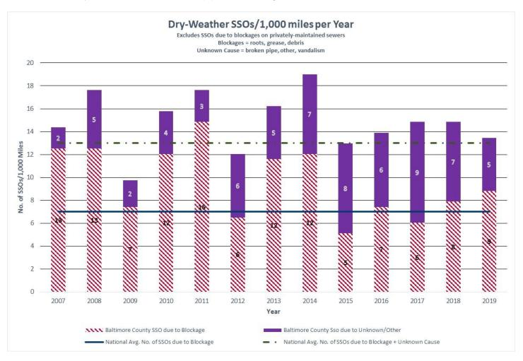
As shown in the above graph, since 2015, the number of SSOs per year due roots, grease and debris is approximately equal to the national average; however, in the same time period, the number of SSOs per year due to unknown/other causes, such as broken pipe, vandalism, etc. has significantly increased compared to the prior 7 year (2007-2014). Since 2015 the total number of SSOs per year has approximately doubled due to unknown/other causes.
