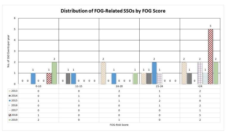
The graph indicates that facilities with a FOG discharge risk score of >16 may have a higher incidence of localized grease-related sewer overflows. The County will further analyze the data to confirm this possible correlation.
